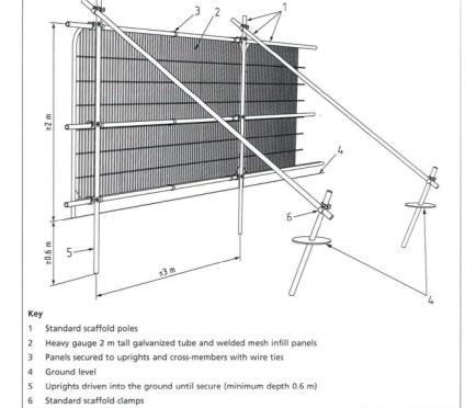
The tree protection fencing is to be erected enclosing the root protection areas around the trees being retained as shown on this drawing and appendix 1\_In some areas, the site hoarding may be sufficient to act as the protective fencing if the tree and its root zone are positioned outside and no works are envisaged within the area outside the site hoarding. This will need to be discussed and agreed at the initial site meeting.
